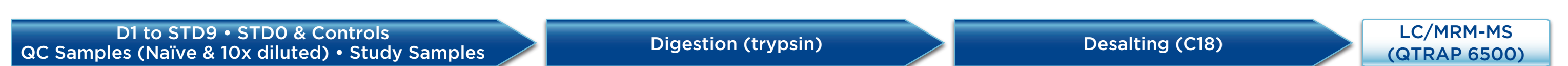
Figure 2. Process flow for Calibration Standards, QC samples, controls and Study samples using heavy-labeled winged peptides.
